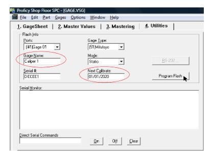
In Version 2.00 of the Wireless Interface Cable, the Gage Type is not programmable for reasons of Flash memory capacity limitations. Since Gage Type is irrelevant to the functioning of the Wireless Interface Cable, the Gage Type defaults to Mitutoyo and is not programmable. If the ability to program the Gage Type is important to you in your application, please let us know at www.kirkwoodcables.com/contact-us.html.
