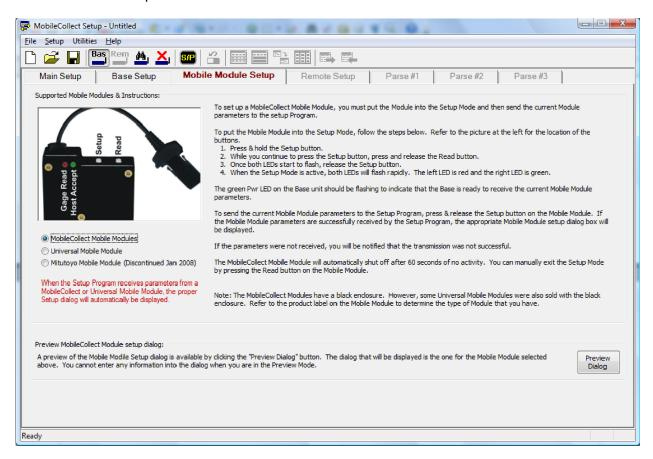
Perform the following steps using the buttons on the Mobile Module to send the Mobile Module parameters to the Setup Program. These steps are also outlined on the Mobile Module Setup tab, although more detail is explained in step #4 below.
