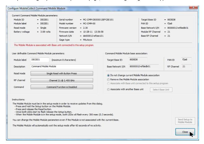
Once this dialog appears, the MobileCollect Setup Program has received the information it needs from this Mobile Module. If the lights on the Mobile Module are still flashing, press and release the Read button to turn them off.
