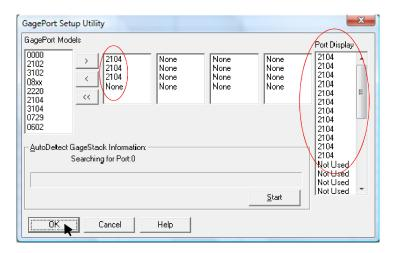
As you can see circled on the left, there have been three 2104 GagePorts detected, and accordingly 12 ports are displayed in the circle on the right. This example shows the results of detecting the 12-port version of the Wireless Interface Cable (2104-3xUSB-GK). If you were to detect the 4-port version of the Wireless Interface Cable (2104-1xUSB-GK), you would see only one 2104 GagePort detected on the left, and only 4 ports accordingly displayed on the right.
